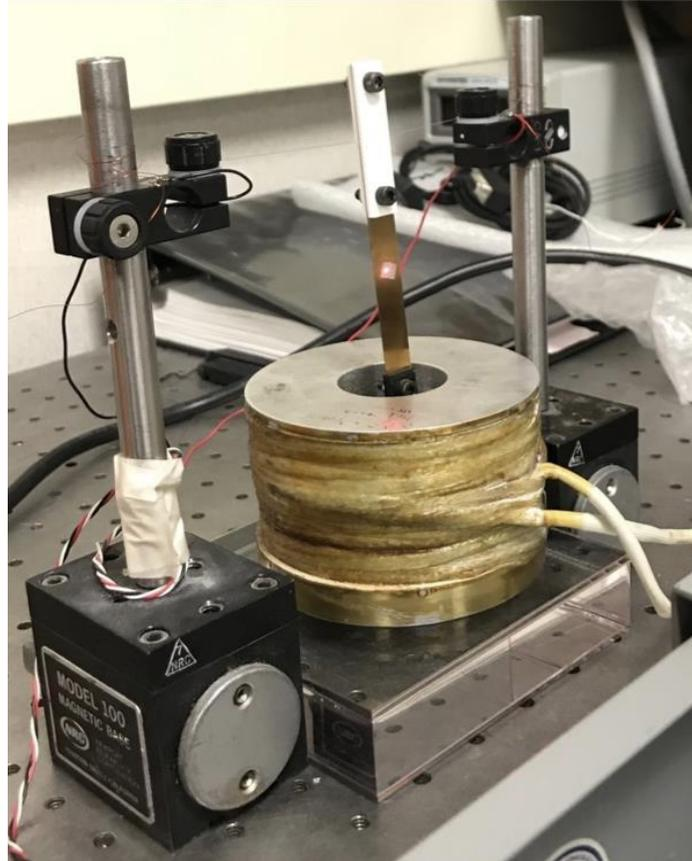
**Figure 1. Free-free fatigue test setup**
